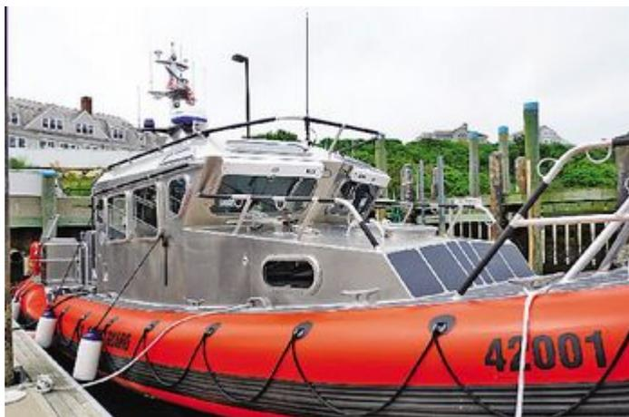
The Coast Guard's state-of-the-art rescue boat will be tethered near the Chatham Fish Pier until crew members complete their training. Steering aboard the vessel is fully computerized and electronic.
