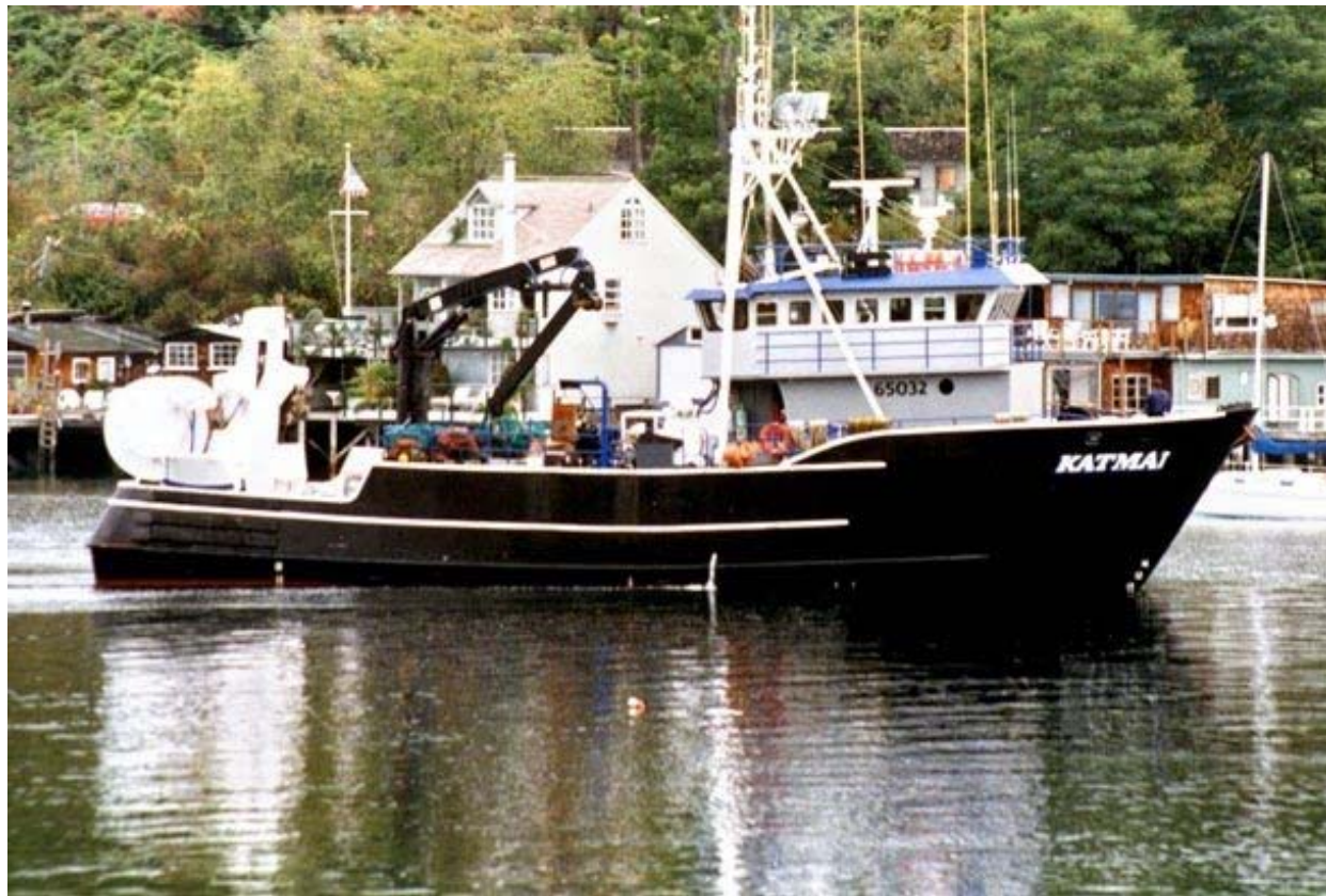
Figure 1. Fishing vessel Katmai motoring through Ballard locks in Seattle (undated Seattle Times photo). White cylindrical structure (net reel) at stern was later removed when vessel was refitted for cod fishing. Katmai was the only vessel owned and operated by Katmai Fisheries, Inc.
