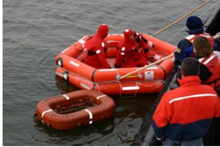
Life float (bottom left) vs inflatable buoyant apparatus (top right)
